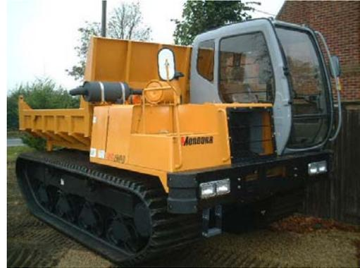
The Morooka Tracked Carrier features a very low ground pressure due to the rocking beam bogey track system. Fitted with a two speed hydrostatic transmission this provides excellent traction and power to the drive motors. The operator can be comfortable working in all climates thanks to the fully air conditioned cab with heater and tinted glass.
